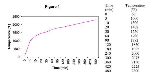
The furnace interior temperature during a test is controlled such that the area under the time temperature curve is within 10% of the corresponding area under the standard time temperature curve for 1 hour or less tests, 7.5% for those less than 2 hours and 5% for those tests of 2 hours or more duration.
