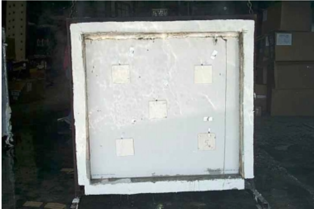
Unexposed surface after the hose stream test
