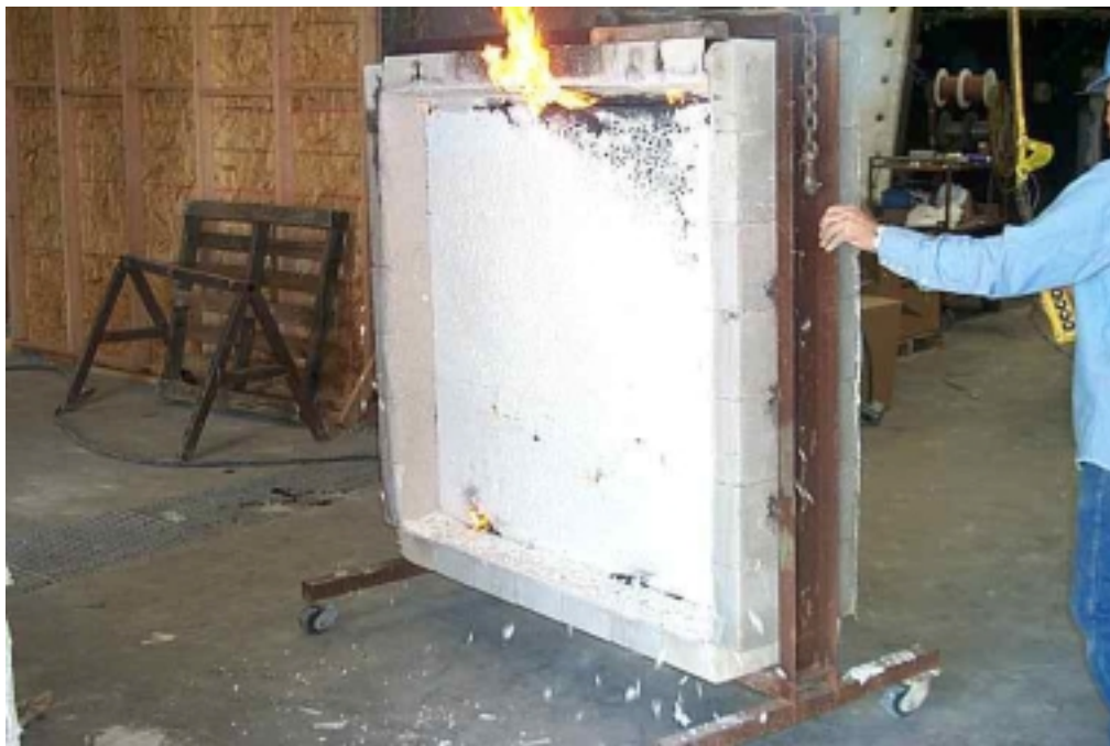
Assembly removed from the furnace and moved into position for the hose stream test
