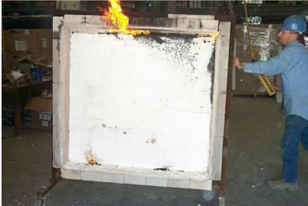
Moving the assembly into position for the hose stream test
