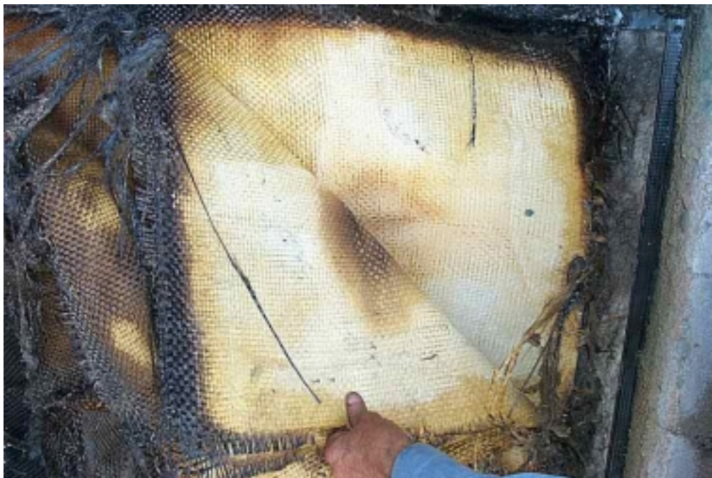
Scorching is seen through 5 of the 17 layers of fabric
